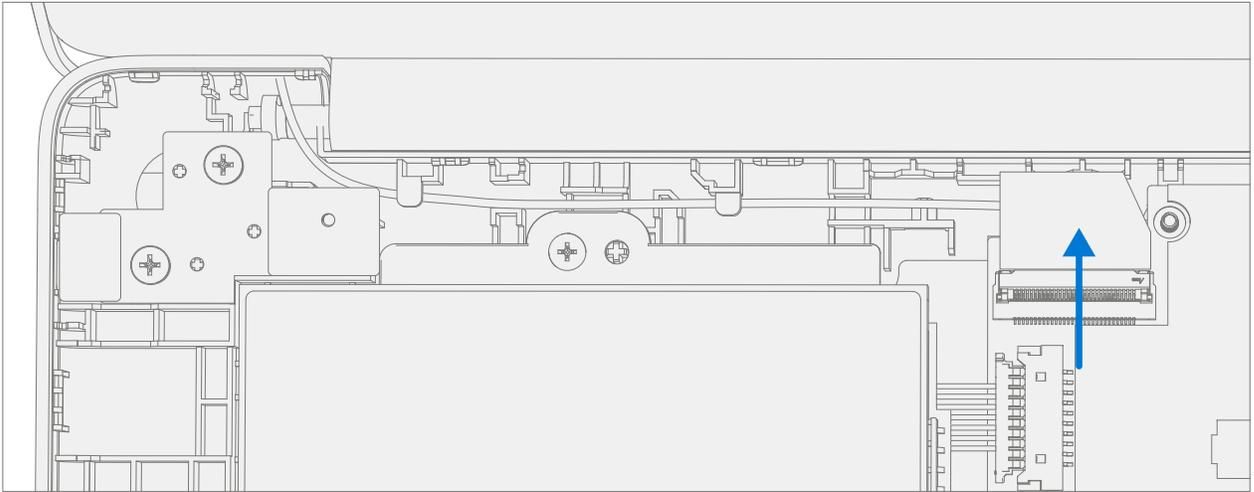
4. **Remove USB Bracket** – Using a PH0 driver remove the two screws from the USB bracket. Remove the bracket from the D-Bucket.
