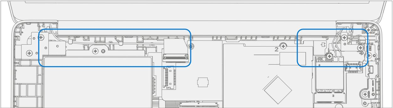
3. **Install New AB-Cover hinge screws** – Using a PH0 driver install two new MS250401060 screws into the left hinge. Install two new MS250401060 screws into the right hinge. Turn all the screws until just snug and seated, and then turn another 45-degrees (1/8 turn) or until fully fastened.
