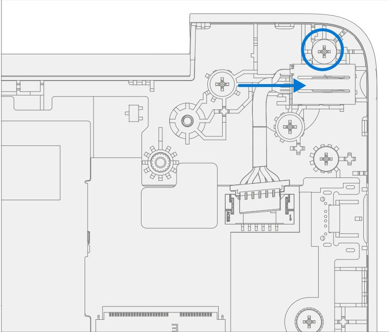
2. **Install USB Bracket** – Place the USB bracket into the D-Bucket. Using a PH0 driver install two new MS20025I070 screws into the USB bracket. Turn all the screws until just snug and seated, and then turn another 45-degrees (1/8 turn) or until fully fastened.
