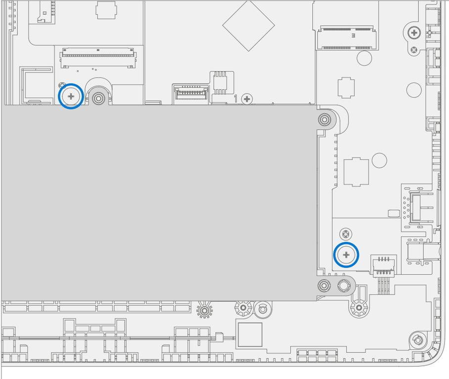
6. **Remove PCBA** – Remove PCBA from the D-Bucket.
