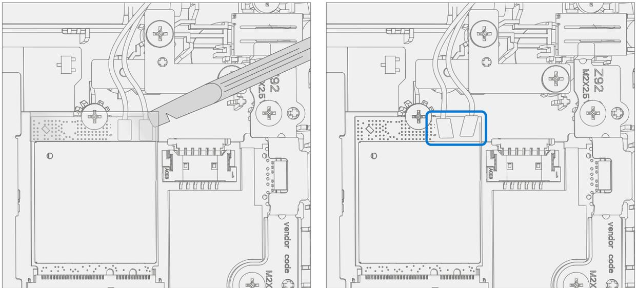
3. **Disconnect AB-Cover Cable** – Using a plastic tool / spudger unlock the AB-Cover cable connector. Remove AB-Cover cable from the PCBA. Carefully remove cable from the D-Bucket channels and hooks.
