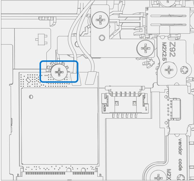
3. **Remove WiFi Module** – Pull the WiFi Module out of the PCBA connector.
