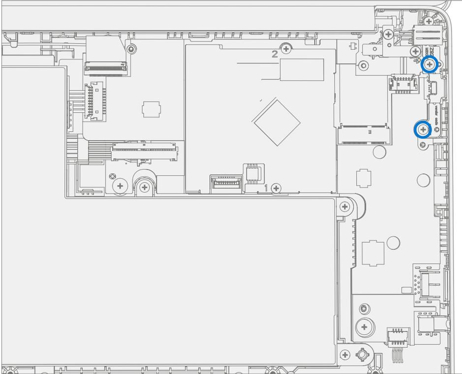
4. **Connect AB-Cover Cable** – Connect the AB-Cover cable into the PCBA. Ensure the cable is fully seated and locked in the connector.
