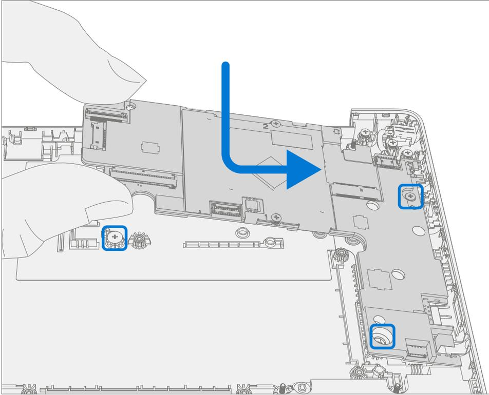
2. **Install New PCBA screws** – Using a PH0 driver install two new MS20015I220 screws into the PCBA. Turn all the screws until just snug and seated, and then turn another 45-degrees (1/8 turn) or until fully fastened.
