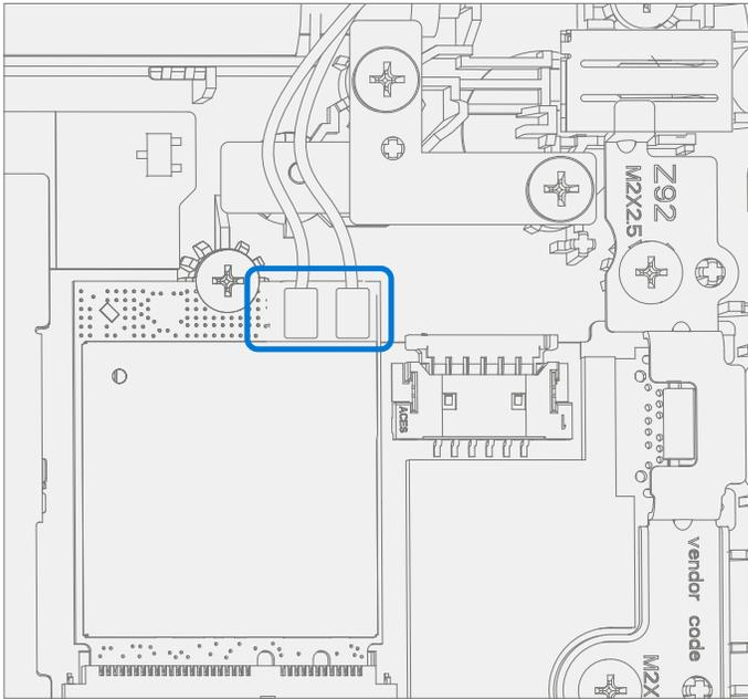
4. **Install Antenna Cable Mylar** – Install a new mylar cover onto the WiFi Module as pictured below.
