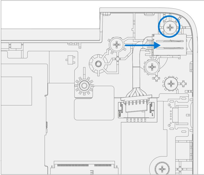
4. **Install USB Bracket** – Place the USB bracket removed from the old D-Bucket into the new D-Bucket. Using a PH0 driver install two new MS20025I070 screws into the USB bracket. Turn all the screws until just snug and seated, and then turn another 45-degrees (1/8 turn) or until fully fastened.
