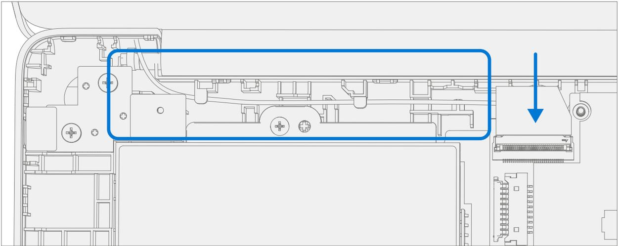
5. **Connect Antenna Cables** – Connect the antenna cables onto the WiFi Module as pictured below. Ensure the white cable is installed on the right side connector and the black cable is installed on the left side connector.
