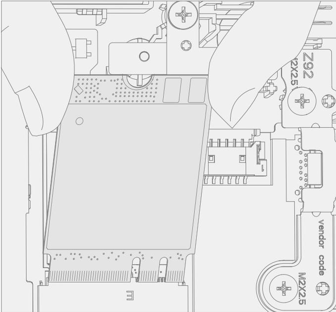
2. **Install New WiFi Module screw** – Using a PH0 driver install a new MS200251070 screw onto the WiFi Module. Turn the screw until just snug and seated, and then turn another 45-degrees (1/8 turn) or until fully fastened.
