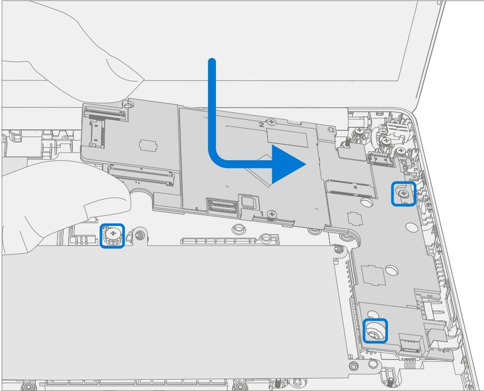
2. **Install New PCBA screws** – Verify the battery, display, antenna, power, and speaker cables are not captured under the PCBA. Using a PH0 driver install two new MS20015I220 screws into the PCBA. Turn all the screws until just snug and seated, and then turn another 45-degrees (1/8 turn) or until fully fastened.
