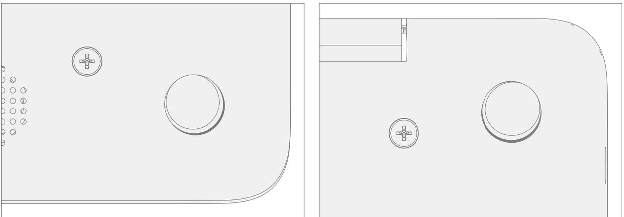
2. **Inspect for anomalies** – Inspect each foot to ensure no cosmetic damage or gaps between the foot and the D-bucket foot recesses exist.
