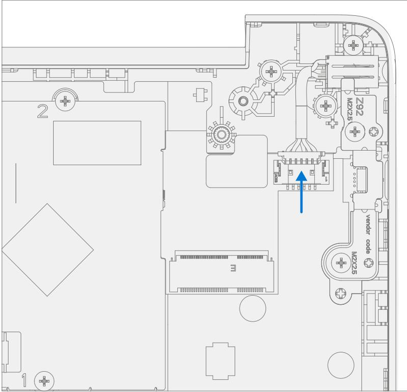
2. **Remove USB Bracket** – Using a PH0 driver remove the two screws from the USB bracket. Remove the bracket from the D-Bucket.
