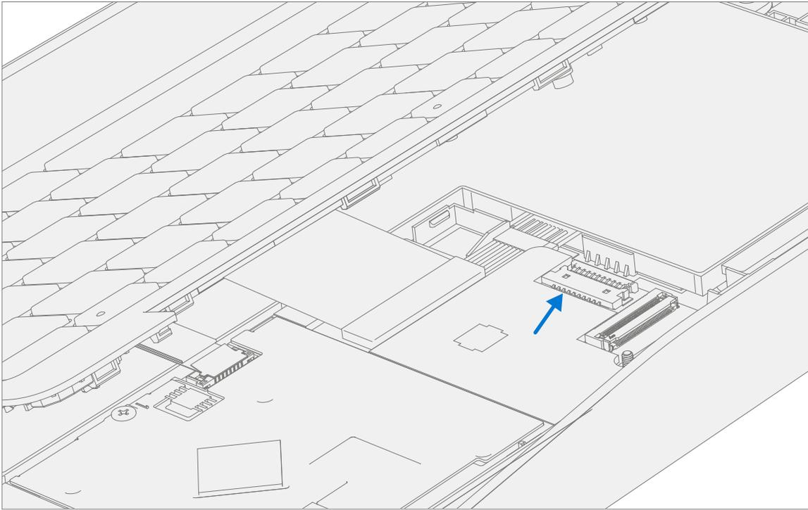
4. **Disconnect C-Cover FPCs** – Holding the C-Cover at an angle use a plastic tool / spudger to disconnect the FPC's from the PCBA.
