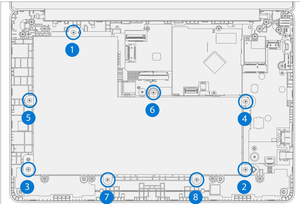
4. **Install C-cover** – Follow steps for Procedure – Installation (C-Cover Keyboard) on [\(page 21\)](#). Leaving C-Cover screws uninstalled.
