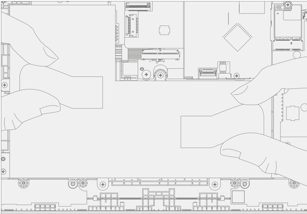
3. **Install New Battery Screws** – Using a PH0 driver install 8 new MS200251070 screws into the battery frame. Follow the installation order pictured below. Turn all screws until just snug and seated, and then turn another 45-degrees (1/8 turn) or until fully fastened. Carefully remove the liner with handling loops.
