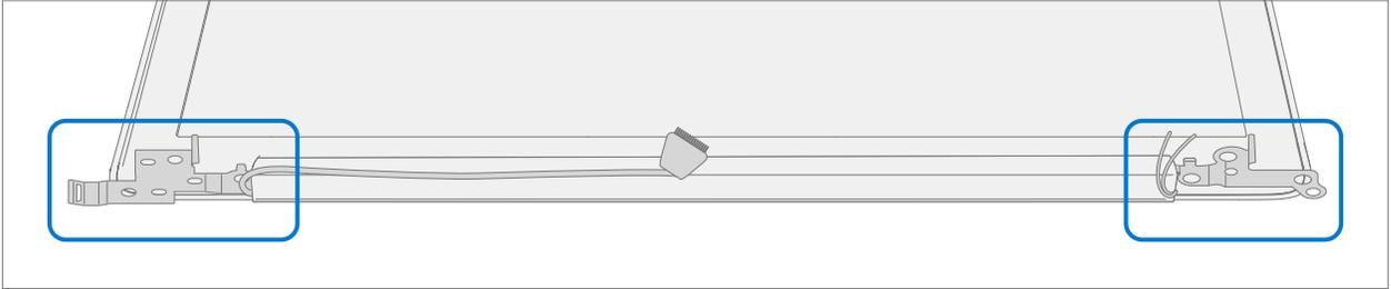
2. **Install New AB-Cover Display Assembly** – Align AB-Cover hinges into the D-Bucket. Ensure display and antenna cables are routed as pictured below.
