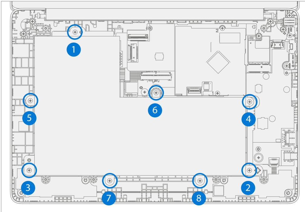
2. **Remove Battery from device** – Carefully remove the battery from the device using two small suction cups.
