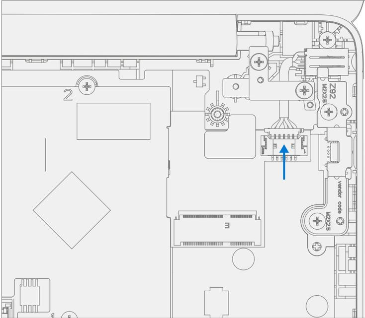
2. **Disconnect Speaker Cable** – Using a plastic tool / spudger disconnect the speaker cable from the PCBA.
