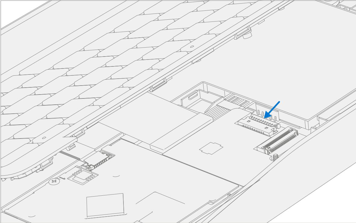
5. **Align the C-Cover** – Properly align the C-Cover to the device using the front edge. Place the C-cover back onto the device. Press down along the outside edges to engage snaps. Press down on the center of the keyboard to engage the keyboard hook.
