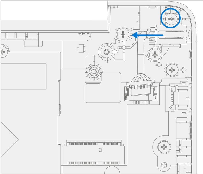
4. **Remove PCBA screws** – Using a PH0 driver remove the two screws from the PCBA.
