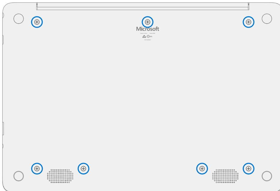
**!** **CAUTION:** All 7 screws must be removed before starting C-Cover removal.
