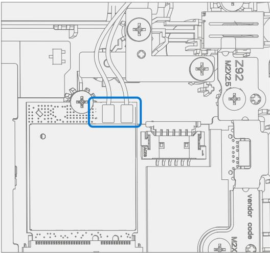
6. **Install Antenna Cable Mylar** – Install a new mylar cover onto the WiFi Module as pictured below.
