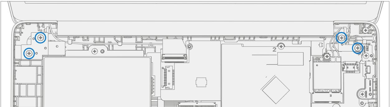
4. **Connect AB-Cover Cable** – Carefully route the cable into the D-Bucket channels and hooks. Connect the AB-Cover cable into the PCBA. Ensure the cable is fully seated and locked in the connector.
