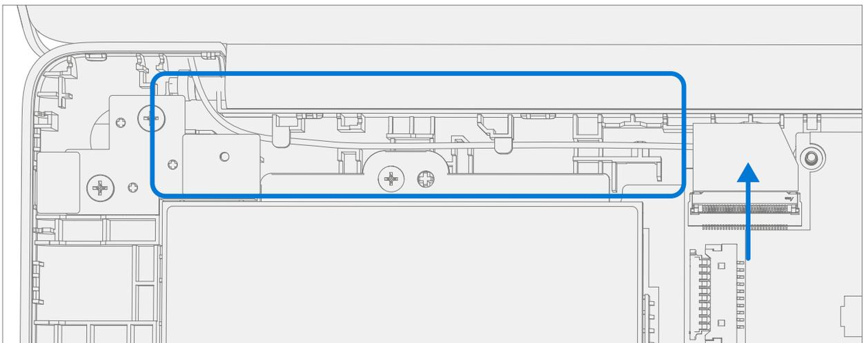
4. **Remove AB-Cover hinge screws** – Using a PH0 driver remove the two screws from the right AB-Cover hinge. While holding the AB-Cover with one hand remove the two screws from the left AB-Cover hinge. Remove the AB-Cover Display Assembly from the D-Bucket.
