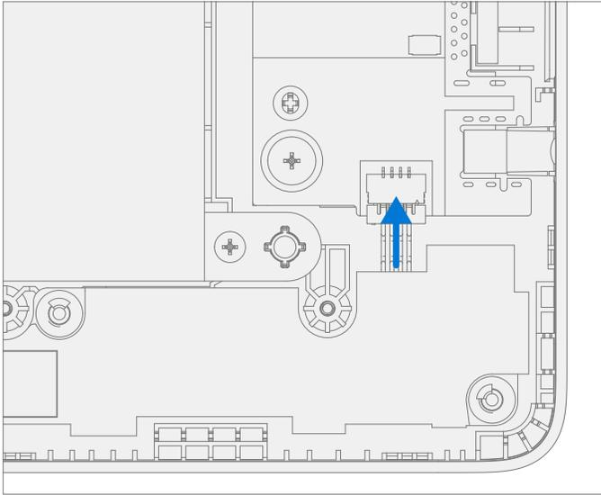
6. **Connect DC Power Cable** – Connect the DC power cable into the PCBA.
