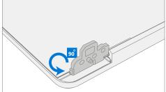
2. **Install display module onto chassis** – While holding the display with one hand. Carefully align the hinges into the pockets on the chassis.
